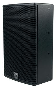
The X10 is a high performance yet very compact two-way passive loudspeaker system which utilises a 10" (250mm)/2.5" (63mm) voice coil LF driver and a 1" (25mm) exit HF compression driver with a 1.4" (35mm) polyimide diaphragm. The rotatable 90° x 50° HF horn has equal horizontal and vertical mouth dimensions for directivity control in both planes.
